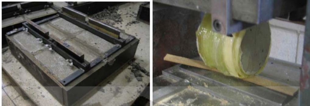
Figure 10. Creation of standardized cracks
