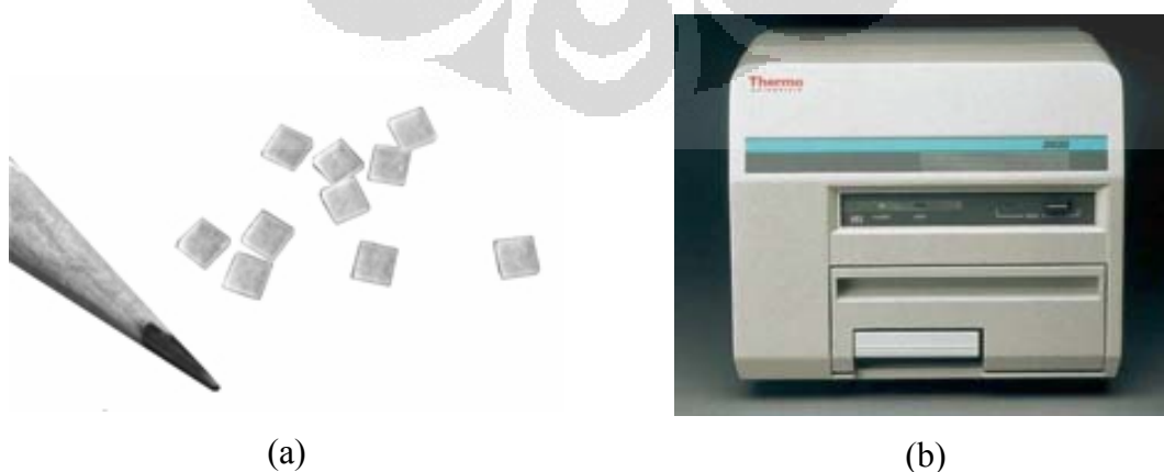
Gambar 2.8. (a) TLD100 chip ; (b) TLD Reader 3500 Harshaw, Thermo Scientific [11]
