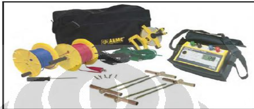
Gambar 3.4 ground earth resistance motor
