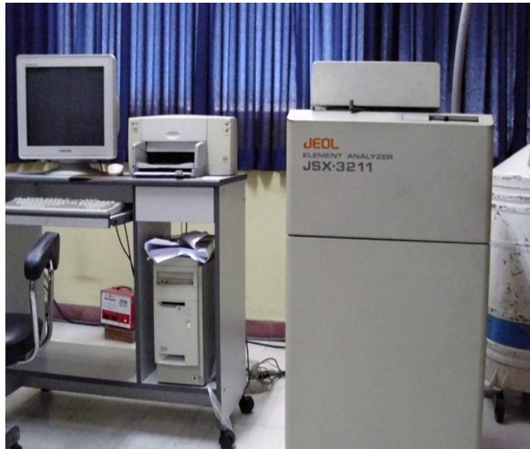
Gambar 2.3 : Alat XRF merk Jeol Element Analyzer JSX – 3211
