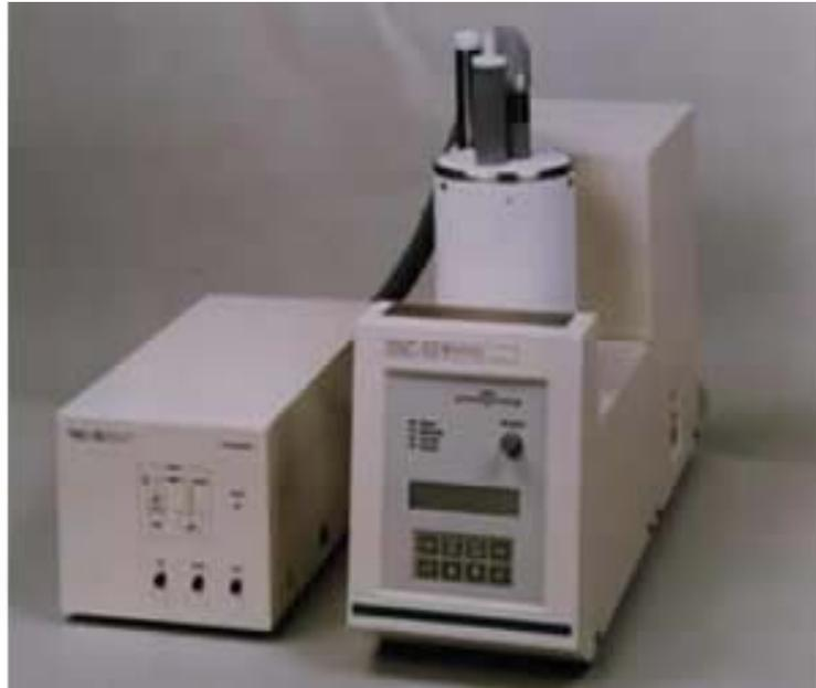
Gambar 2.7 : Differential Scanning Calorimeter ( DSC ) merk Shimadzu tipe 50
