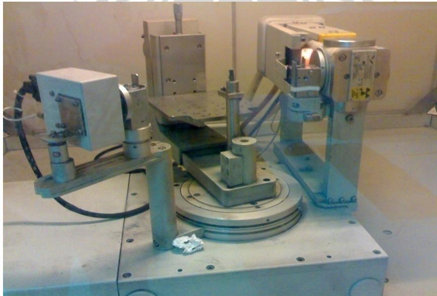
Gambar 2.6 : X-Ray Powder Diffractometer ( XRD ) Philips PW 3710/40kv
