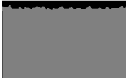
Gambar 2-5. Korosi merata ( http://www.poeton.co.uk/w1/images/corrosion/general.gif )
