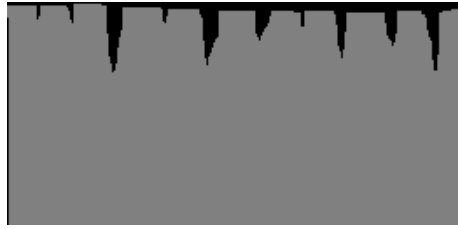
Gambar 2-6. Korosi sumuran. ( http://www.poeton.co.uk/w1/images/corrosion/pitting.gif )
