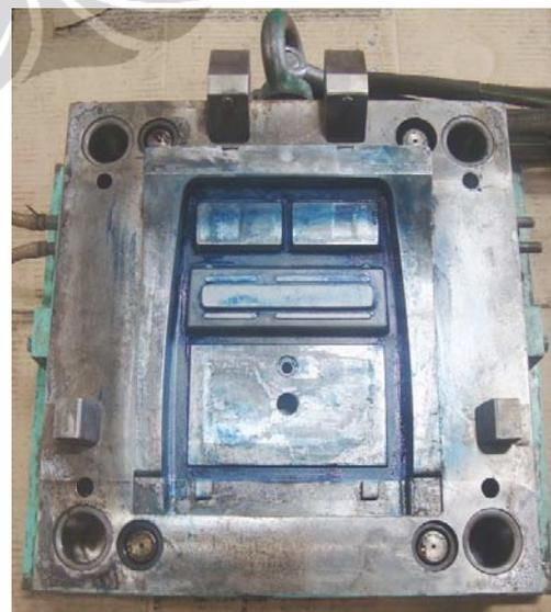
Gambar 8b. Cavity Plate
