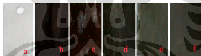
Gambar 4.9: Uraian rendaman kupon: (a). sebelum direndam, (b). 0 mL, (c). 1 mL, (d). 2 mL, (e). 3 mL, (f). 4 mL
