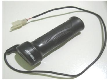
Gambar 3.2. Handel Akselerator
