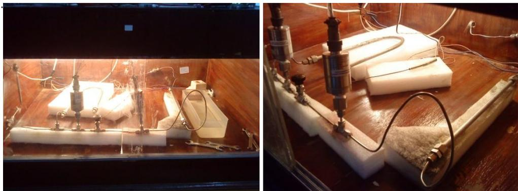
**Gambar 3.3** Alat Uji Adsorpsi
