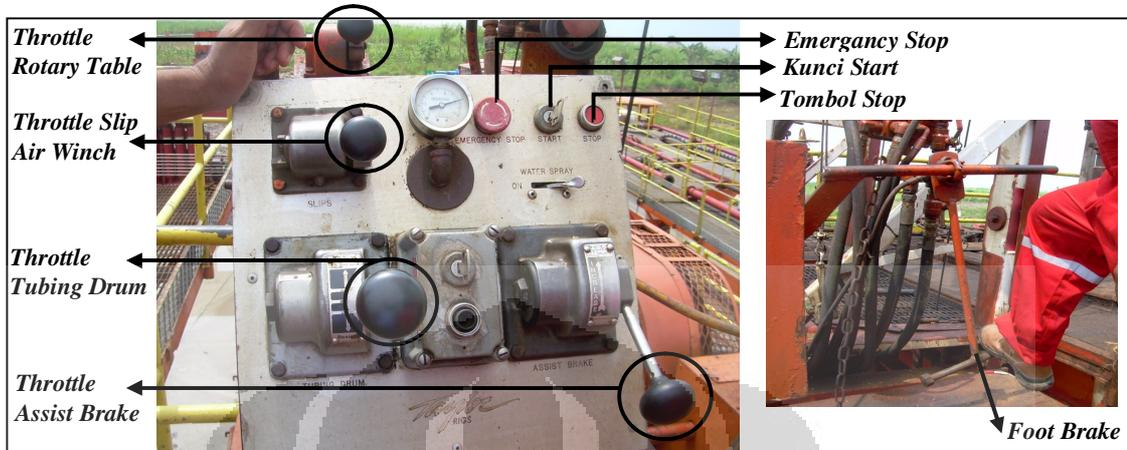
**Gambar 5.4. Control Panel Console dan Foot Brake**
