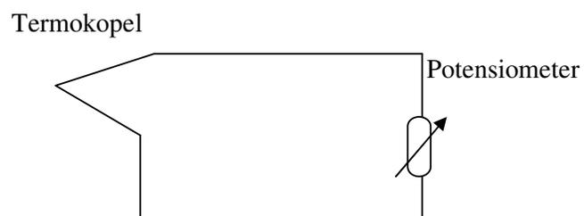
Gambar 3.5 Rangkaian Termokopel Dengan Potensiometer
