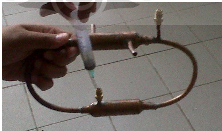
Gambar 3.8 Pengisian fluida loop heat pipe .
