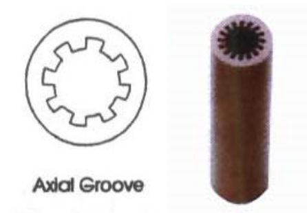
Gambar 2.5 Axial groove wick [29]
