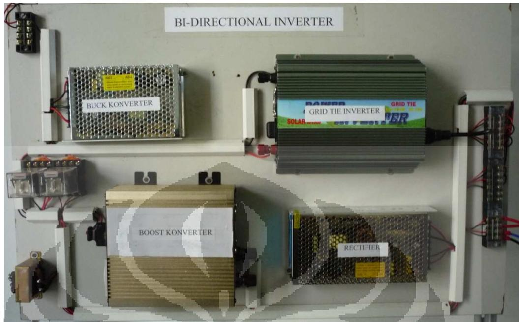
Gambar Konfigurasi Bi-directional inverter
