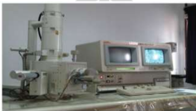
Gambar 3.5. Alat Uji SEM (Scanning Electron Microscope) JEOL JSM-5310 LV
