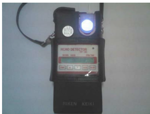
Gambar 5.19 Riken Keiki FP30 Formaldehyde Detector
