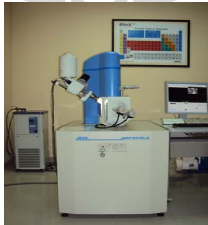
Gambar 4.7 Alat Scanning Electron Microscopy (JEOL JSM 6510LA)
