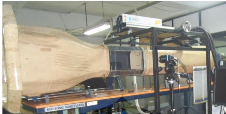
Gambar 3.14 *Sub sonic wind tunnel* Armfield C2-00
