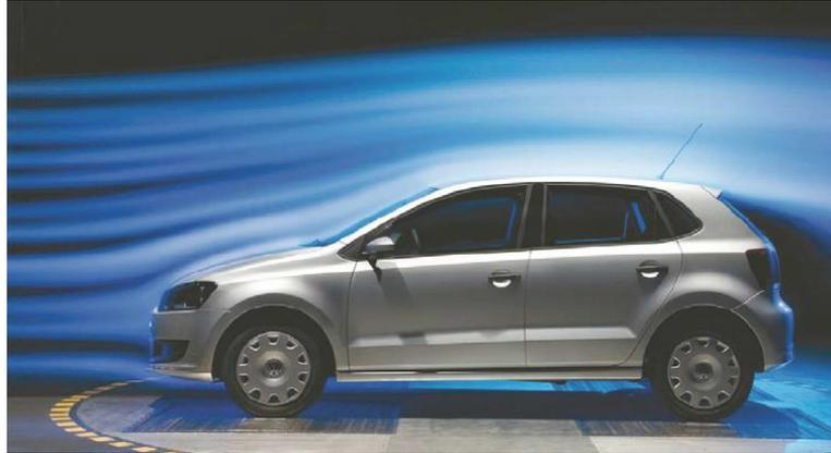
Gambar 2.2 Pola aliran udara disekitar kendaraan ([www.carbodydesign.com](http://www.carbodydesign.com))
