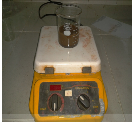
Gambar 3.5 Proses Pelindian Laboratorium Korosi DMM
