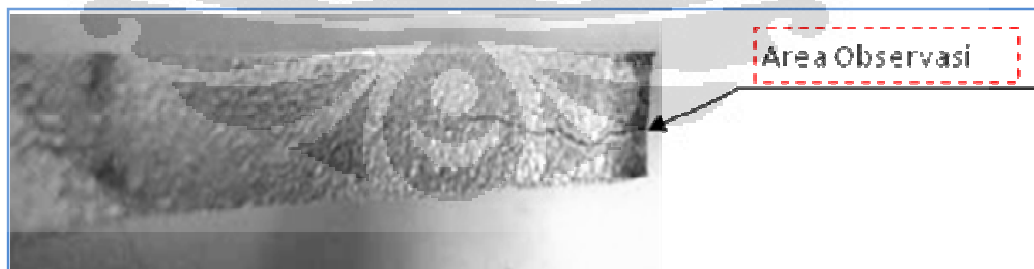
Gambar 4.7 Area pengamatan SEM cylinder head retak
