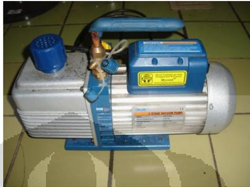
Gambar 3.17 Pompa Vakum
