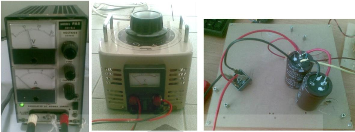
Gambar 3-11. DC Supply, AC Supply, dan Rectifier
