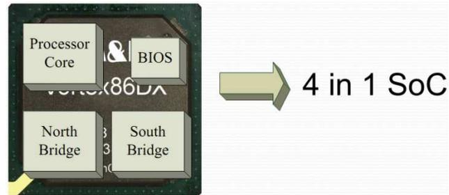
Gambar 2.8. Vortex86DX Single On Chip (SoC)
