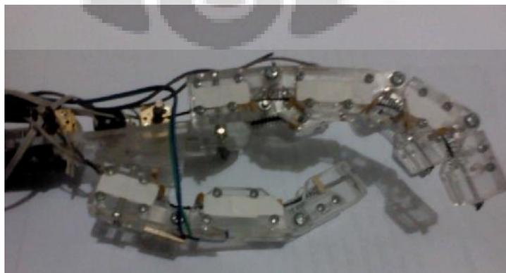
*Gambar 3.3. Gambar Asli Telapak Tangan Robot*
