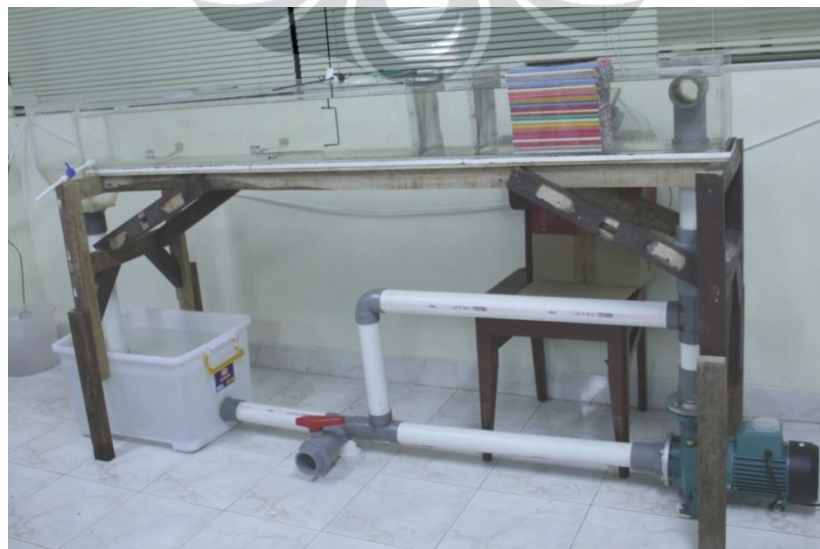
Gambar 4.1 Terowongan air / water tunnel
