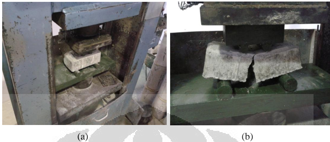
Gambar 11. (a) Pengujian Kuat Lentur Sampel Paving Block
