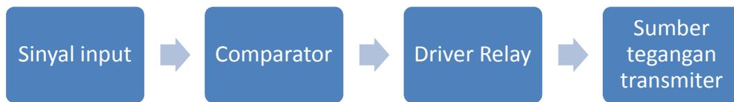
Gambar 3.13 Blok diagram rangkaian switch relay otomatis
