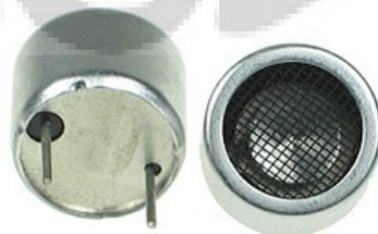
Gambar 3.12 Sensor Ultrasonik
