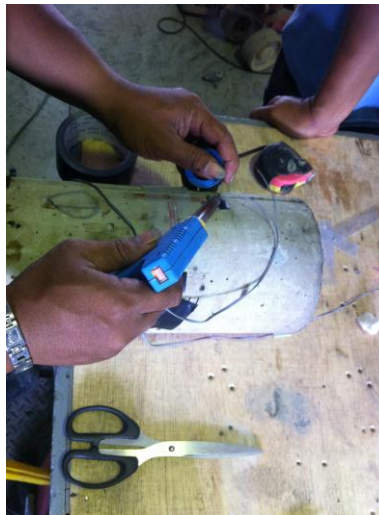
Gambar 4.22 Proses Pen-solderan Kabel ke Stain Gauge
