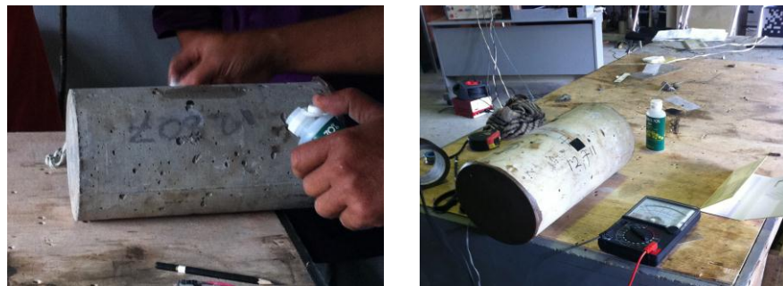
Gambar 4.21 Proses Pemasangan Strain Gauge
