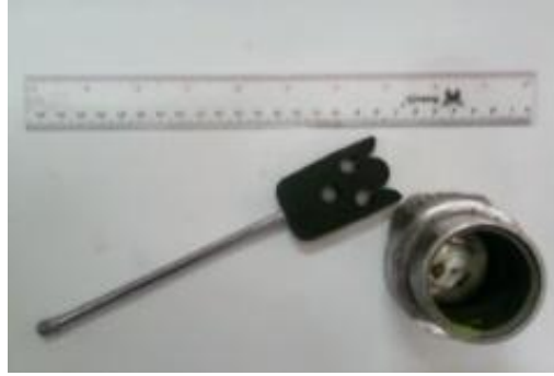
Gambar 3.5 Alat Uji Mulur
