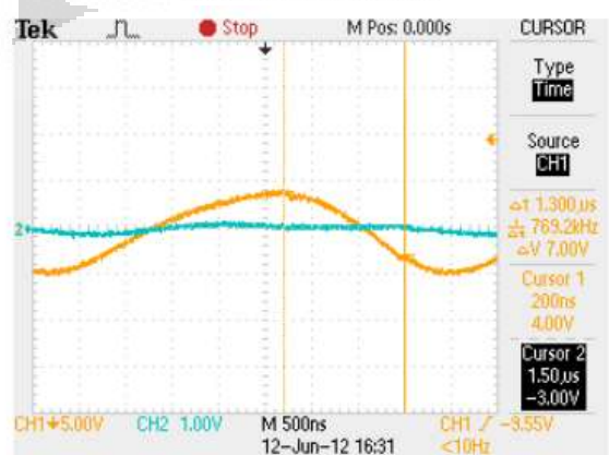
Delay Time Triangle 220 kHz
