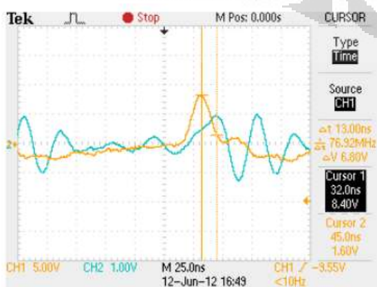
Delay Time Triangle 5 MHz
