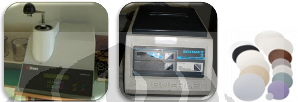
Gambar 3. 9. (kiri-kanan) Hot Mounting – Mesin amplas/poles – amplas & kain poles halus
