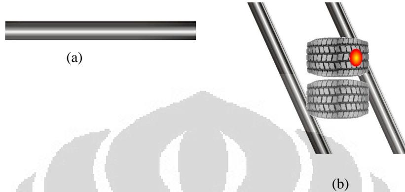
Gambar 2.18(a) Treadle axle counting; (b) Double wheel detection treadle [5]
