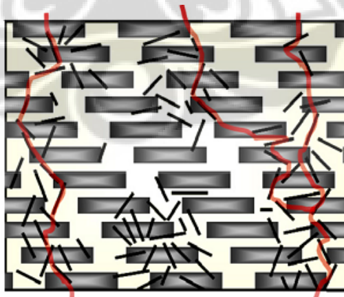
Gambar 2.16 Aglomerasi multi-walled carbon nanotube [28]
