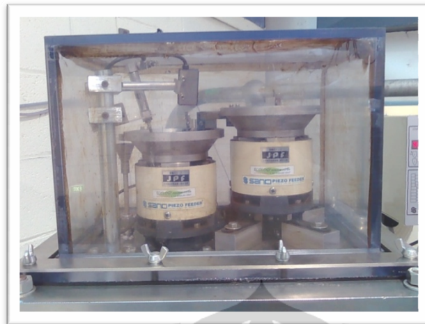
Figure 3.2.1.4 Hopper at the top of the reactor after closing the lid
