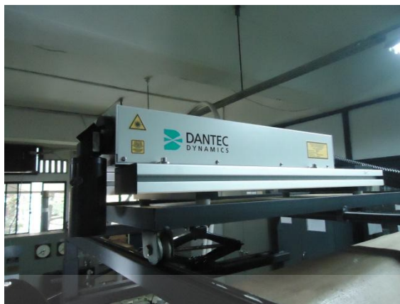
Gambar 3.8 double-cavity Nd:YAG laser
