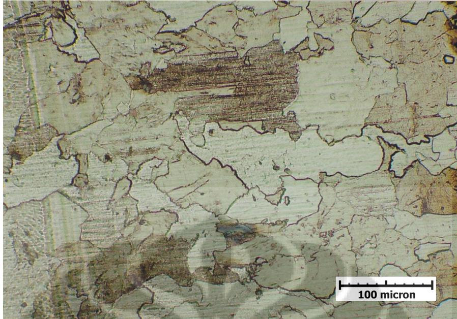
**Gambar 4.17** Struktur HAZ TS 2 kA. Nital 2-3%, 200x
