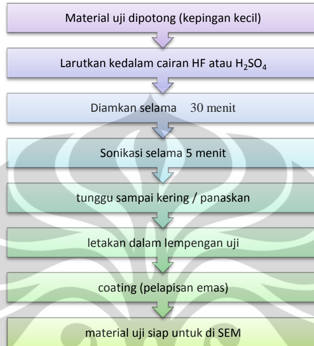
Gambar 3.10 : Diagram alur proses etsa material
