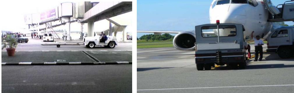
Gambar 5.1.f ATN di service road dan persiapan push back,
