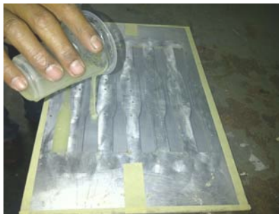
Gambar 3.2. Proses Casting Epoxy Resin
