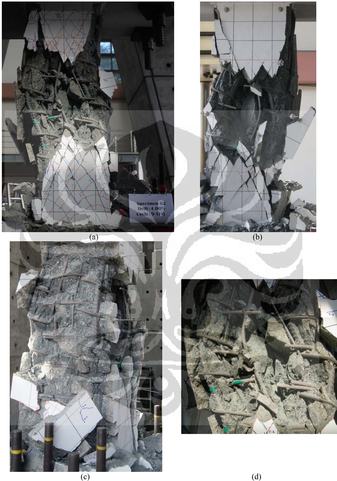
Figure 5.49 Final stage of column S2 (4.00 % drift ratio). (a) West side; (b) East side; (c) South-east side; (d) Failure of large spiral transverse reinforcement at the mid-height of the column west side.
