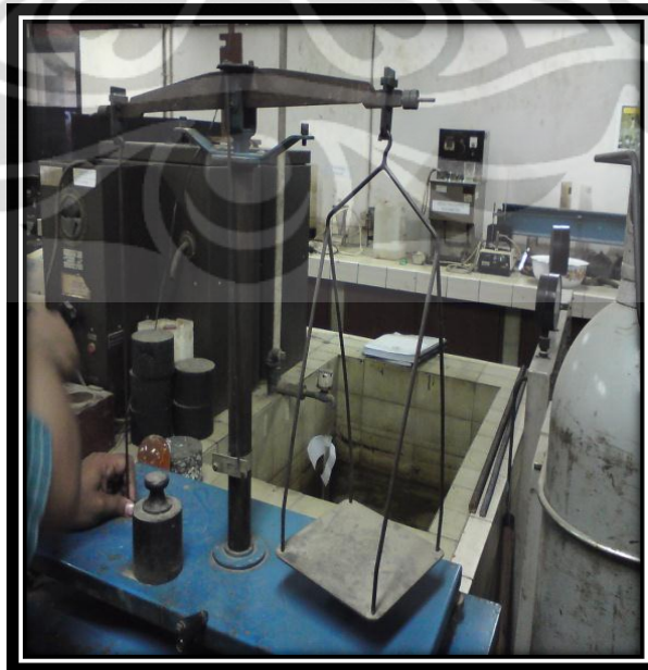
Gambar 3.5. Penimbangan agregat didalam air.
