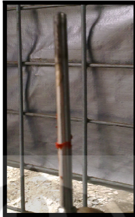
Gambar 4.4 Termokopel gas produser sesudah gas cleaner
