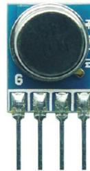
**Gambar 2.10.** *Transmitter TWS-434A*
