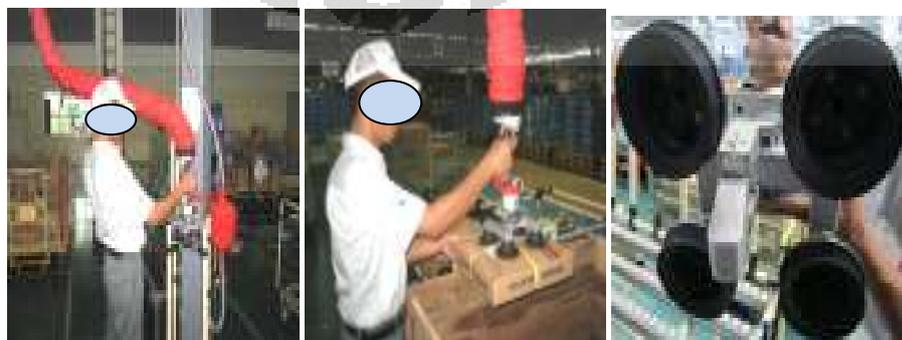
Gambar 7.1 Alat Bantu *Vacuum Lifter* Di *Line Finish Good*
