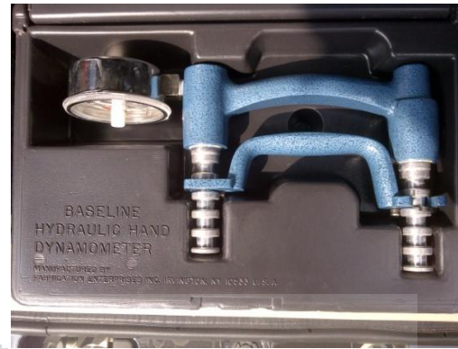
Gambar 2.5 Hand-Grip Dynamometer (tampak samping)
