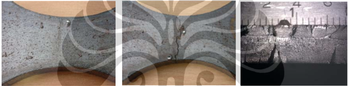
Gambar L.2 Hasil uji fatigue – spatter
