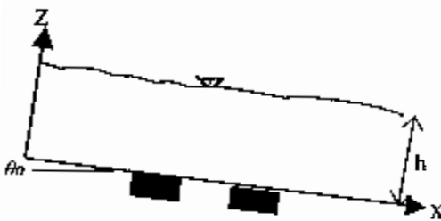
Figure 1. Schematic diagram of gravity flow of a sand-mixture
