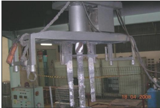
Gambar 3.2 Mesin Gas Buble Floatation
