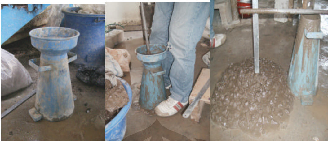
Proses pengujian slump
