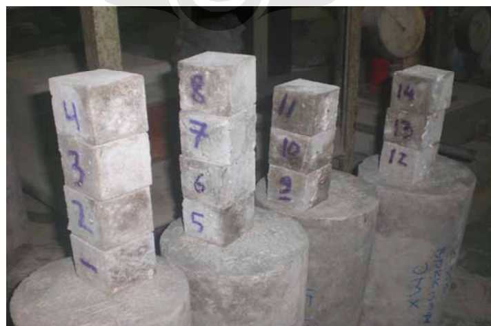
Sampel Kubus (5x5x5) cm Beton Ringan
